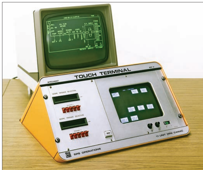
The Touch Terminal as developed for the Antiproton Accumulator (AA).
