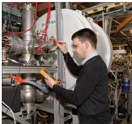
Michael Block, head of the research team, sets up the ion trap SHIPTRAP at GSI, which uses a double Penning trap system. (Courtesy G Otto/GSI.)
